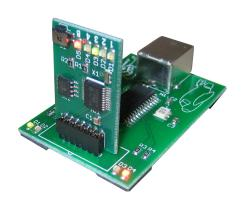
This device allows you to read data from your Futaba-based memory modules and view, edit, save, and write back data using your personal computer. You can also easily email the data to a friend so he/she can load it onto their radio.
