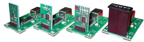
If you have a **CAMPac** made by Futaba then it will plug in with the label facing away from you. Also notice the alignment groove on the plastic casing will correspond to the white outline on the interface. Do not shift the module one pin to the left or right.
