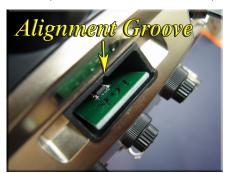
shifted one pin to the left or right. Take care not to install the module incorrectly, as this could result in damage to the  $HH\ 16K\ Memory\ Module$  and/or your transmitter.
