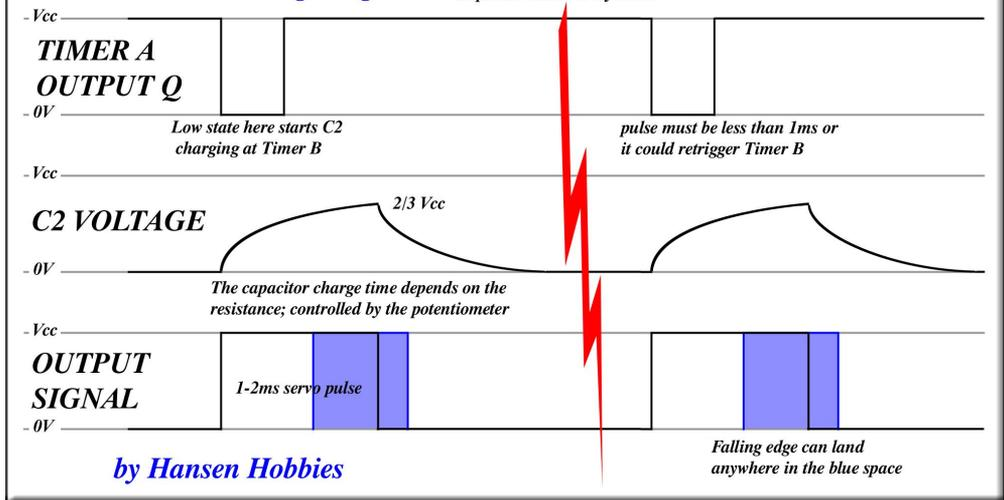
**P1** is a **10K $\Omega$**  potentiometer that can be anything from **0** to **10K $\Omega$** . When you plug in values of **0-10K $\Omega$** , **10K $\Omega$** , and **0.1 $\mu$ F** for **P1**, **R3**, and **C2**, respectively, we get results of **.001 through .002**, exactly the **1-2ms** needed for the PWM.
